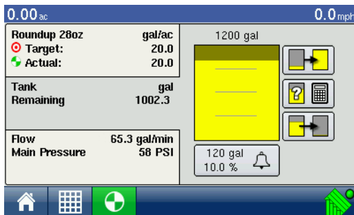
Container (Shown Partially Full)
